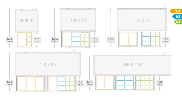
Note: even though drawer capacity of some TRCB units may appear to accept a larger than **1/1** GN pan, the drawer construction of these units are moulded specifically for this pan size as a way of strengthening the drawer and durability of the product.
